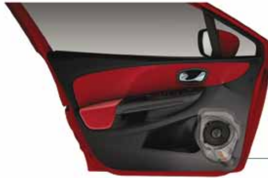
INTEGRATION of a vented loudspeaker in the door of Clio IV
